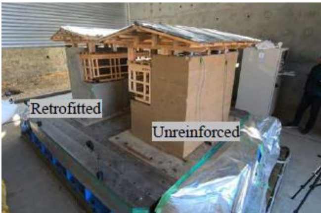
Specimens on shaking table (above). Location of accelerometer sensors (below).
