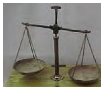
A beam balance: used to measure the mass of an object.
